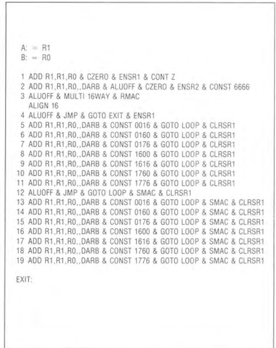
Figure 34. BCD Add Microcode.
